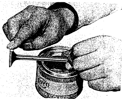
Fig. 3-70 Applying lapping compound to valve face
