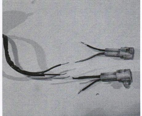
Match black to black and black/white or red to black/white or red when wiring your plug to the new pump. Heat shrink wire connectors provided (just use a lighter to
