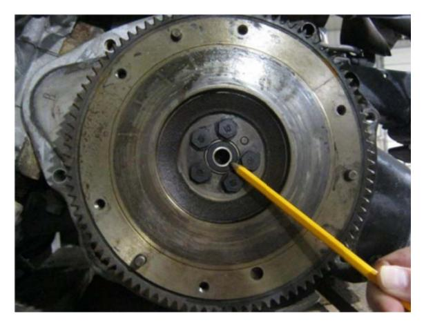
2. Inspect the transmission spline for wear and damage. Clean and apply lube, but **<u>do not over</u> <u>lube</u>**.
