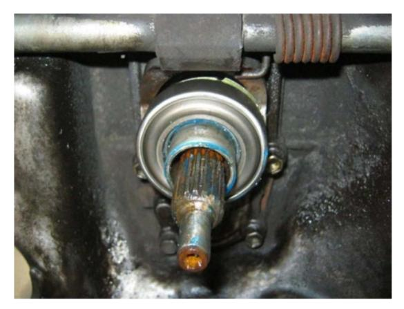
4. Inspect the clutch arm assembly. Clean and lube the bearings on each end. Pull the clutch cable and ensure the clutch arm assembly operates smoothly and returns to its original position.
