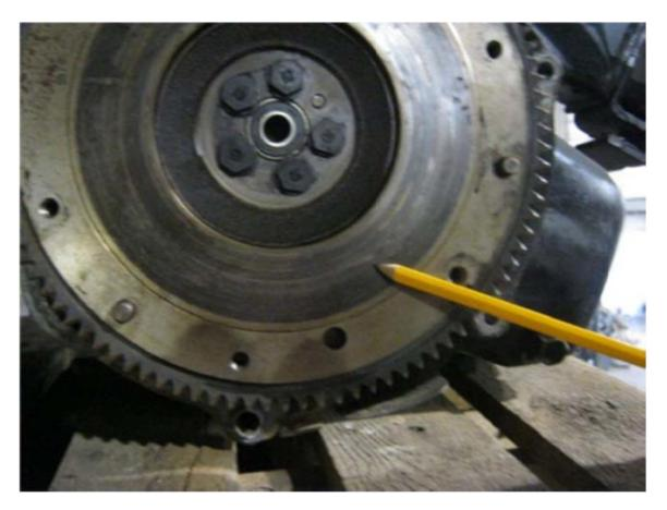
If teeth are chipped or missing you should replace the flywheel.
