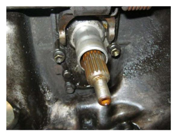
3. Inspect the surface the throw out bearing rides on. Clean and lube.
